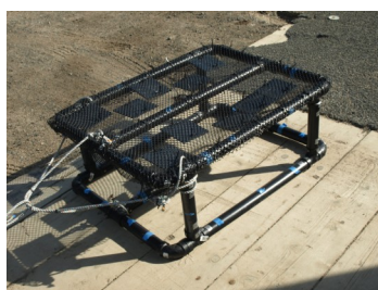
Sled designed for polar sampling. Photo: Gary Freitag
